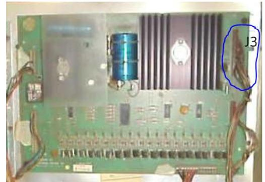
With your multi-meter, set to DCV measurement. Place the black test lead on the GND test-point and using the red test lead check each one of the other test-points. Voltages measured should be +/- 2V, with the exception of the +230V, which could be +/- 10V.
